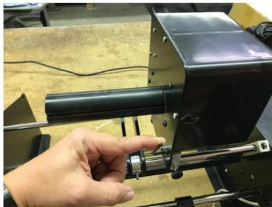
Place Rewinder into position, aligning slots in side frame with rods. Rotate mounting blocks so that holes in mounting blocks align with holes in Rewinder side frame. Insert screws through re-winder side frame and into mounting blocks. Tighten with provided allen key. To move side to side on machine, simply loosen thumb screws in mounting blocks, relocate and then re-tighten.
